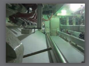
Valves in the maintenance/retracted position with nozzles suspended over the maintenance tray
