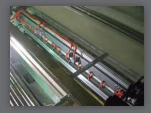
Adhesive manifold and valve assemblies mounted inside tissue machine
